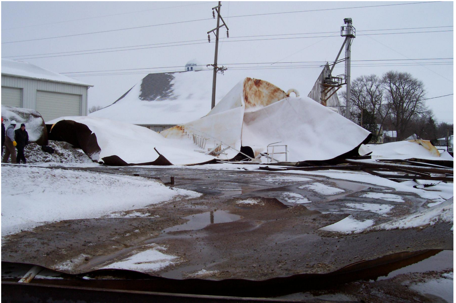
Weld seam rupture. Force of rupture “pushes back”. Rupture on side of camera location.
