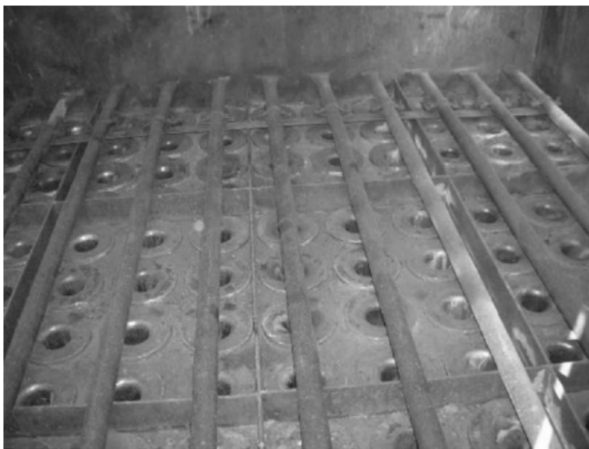
Figure 5.16. Tube sheet of dust collector, Ref. 5.25.
