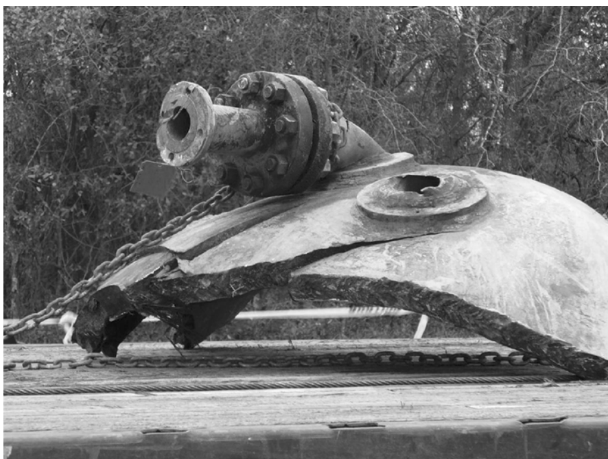
Figure 5.24. Portion of 3 inch thick reactor, Ref. 5.28.
