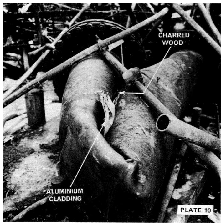
Figure 3.24. The collapsed 20 inch pipe.
