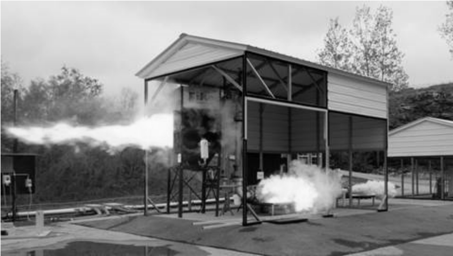
Figure 5.20. Dust collector explosion venting, courtesy Fike.
