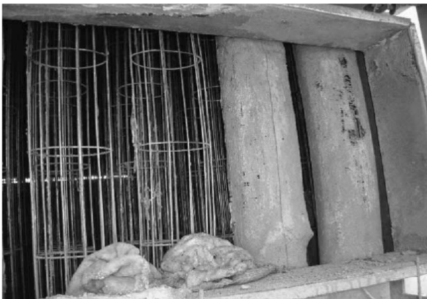
Figure 5.15. Damage to dust collector bags, Ref. 5.25
