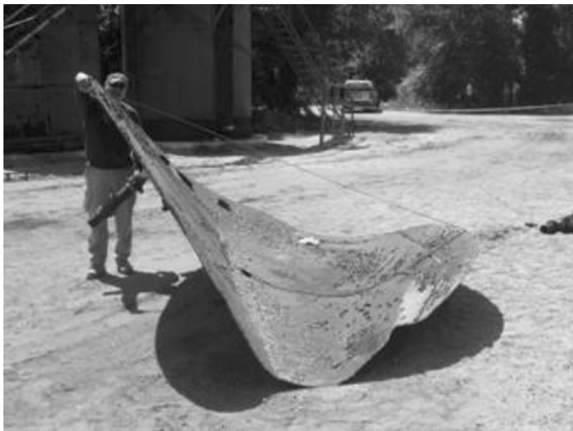
Figure 3.17. Tank 3 lid, source (CSB, 2007).
