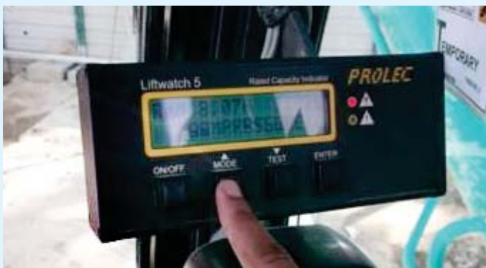
Indicator with working radius and corresponding SWL
